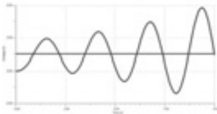
Figure 40. Transient response of the OA implementation of the system - K = 20 .
